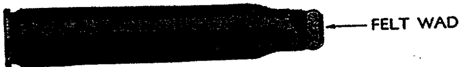
FIGURE 18.—Blank cartridges—necks in section showing wads.
